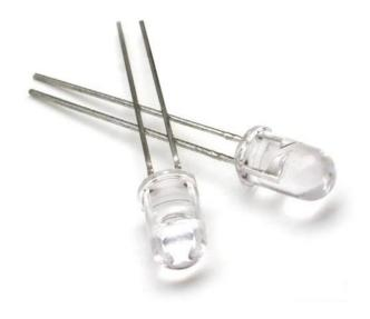
In the image above you are able to see an infrared LED that is an Infrared "Light" Emitting Diode. These LED's are widely used in remote controls for TVs, DVD players, etc... When you point your remote control to your TV and press a button your infrared LED with "light".
